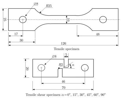
Fig. 1. Uniaxial tension test specimens
