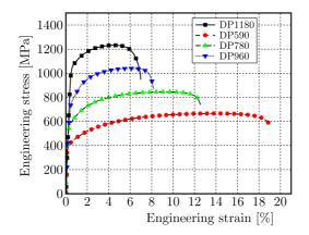
Fig. 2. Engineering stress-strain curve of dual-phase (DP) steel
