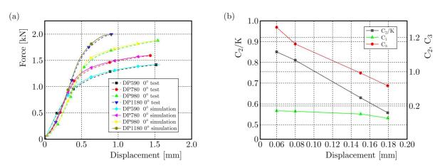
Fig. 5. (a) Comparison of load-displacement responses of simulations with 0° shear specimen against experimental data. (b) MMC parameters curve
