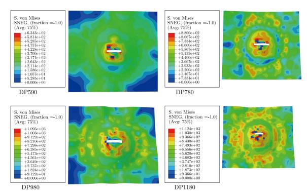
Fig. 12. Nakazima model fracture simulation
