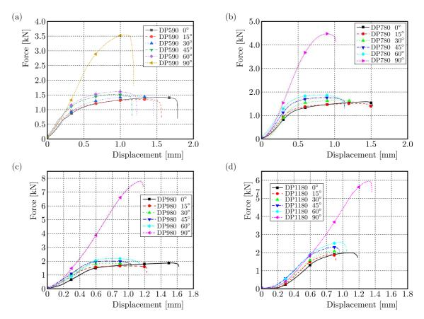
Fig. 3. Load-displacement curves of shear tests
