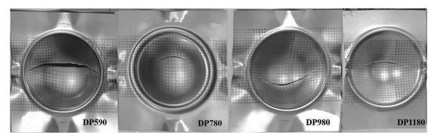
Fig. 11. Nakazima test specimens
