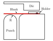
Fig. 10. Nakazima test punching machine mould
