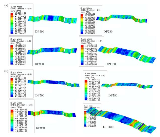
Fig. 9. Stretch-bending model fracture simulation
