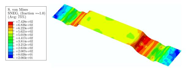
Fig. 7. Unbroken stretch-bending simulation
