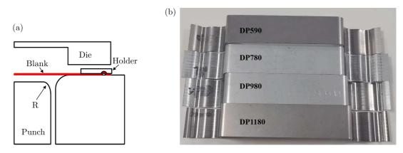
Fig. 6. (a) Punching machine mould. (b) Unbroken stretch-bending tests
