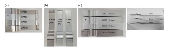
Fig. 8. Fractured stretch-bending specimens
